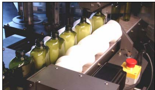
Model 2000NR Feedscrew Infeed
