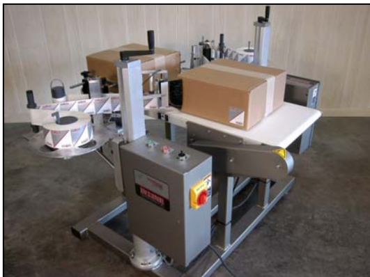
680 Pressure Sensitive Case Labeler showing two-label application.
